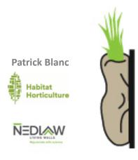
Synthetic felt attached to a support structure. All felt systems are planted onsite.
