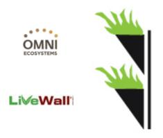
A support structure is erected that holds a series of planting units. This category is very similar to Tray systems but each planting unit isn't segmented. Containers also use an engineered soilless mix.
